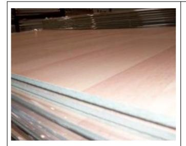
Figure 3: Finished product (Melamine faced MDF boards)
